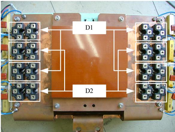
Fig. 7. Photograph of final rectifying stage and secondary copper plate.
