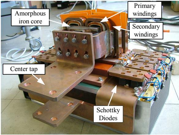
Fig. 6. Photograph of transformer and final rectifying stage.
