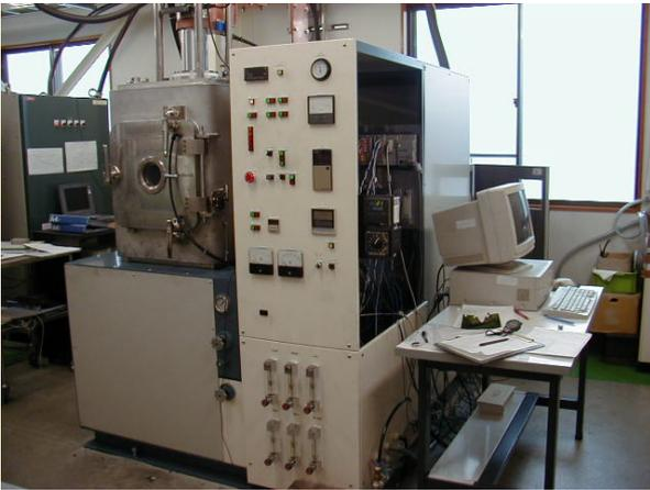
Fig. 1. Overview of sintering system.
