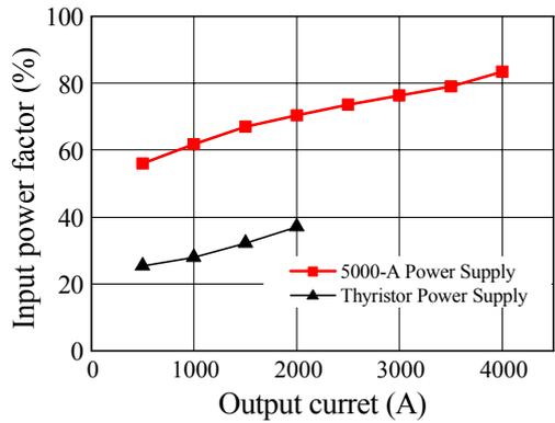
Fig. 10. Total input power factor on utility power source side.
