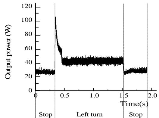
Fig. 8 Output power of PEM fuel cell (Left turn)
