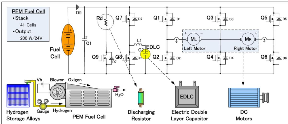
**Fig. 4** Control of energy flow and motor drive circuit
