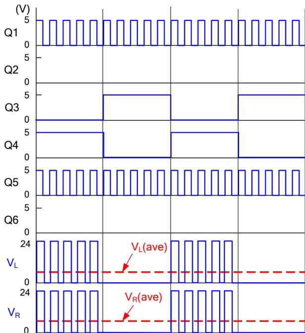
**Fig. 10** Waveforms of DC chopper (Forward)
