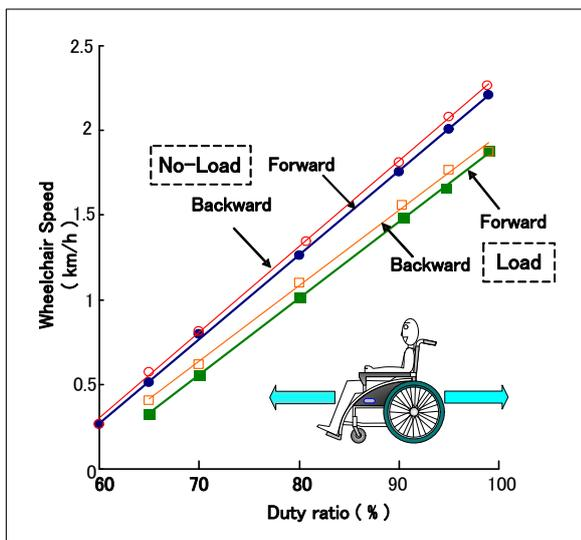
**Fig. 11** Wheelchair speed to switching duty ratio
