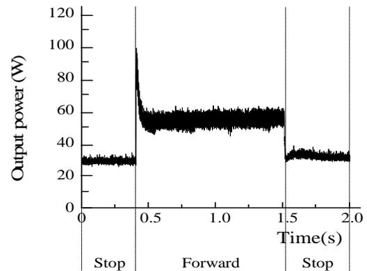
Fig. 7 Output power of PEM fuel cell (Forward)
