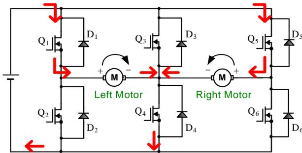
**Fig. 9** Operation of DC chopper (Forward)
