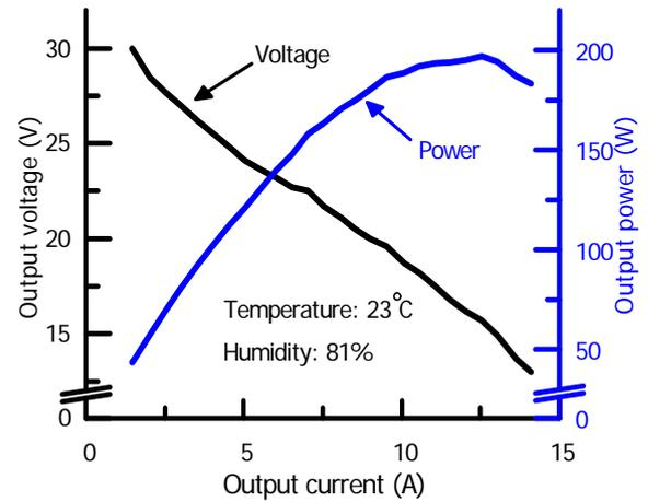
Fig. 6 Characteristics of PEM fuel cell
