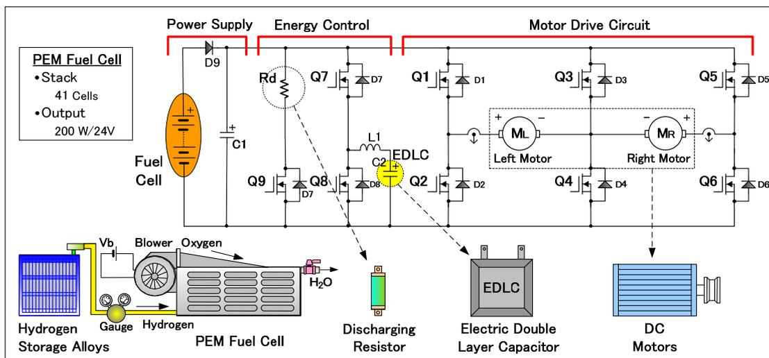
Fig. 3. Management of energy flow and the motor drive circuit.
