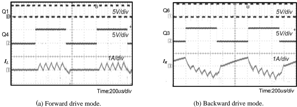
Fig. 8. Experimental data of the improved three-leg full-bridge DC chopper.
