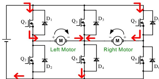
Fig. 5. Operation of the four-quadrant DC chopper (forward drive mode).
