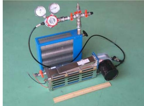
Fig. 2. PEM fuel cell and hydrogen storage alloys.
