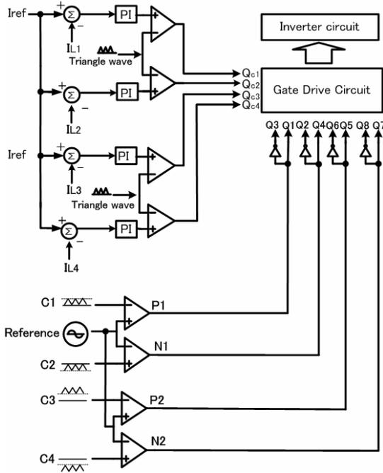
Fig. 11. Controller diagram of five-level CSI
