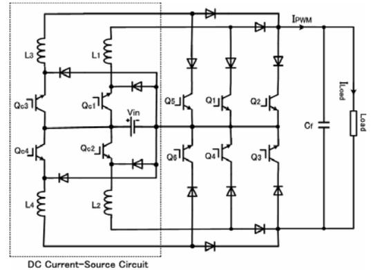
Fig. 9. Simulation and experimental test circuit of five-level CSI
