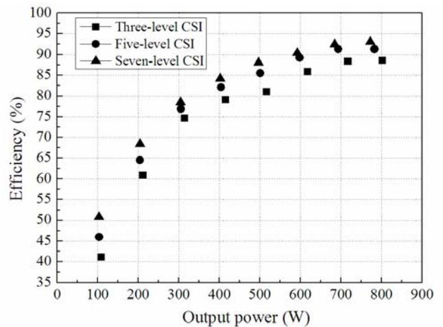
Fig. 14. Efficiency characteristics of proposed multi-level CSIs
