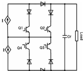
Fig. 1. Fundamental three-level CSI
