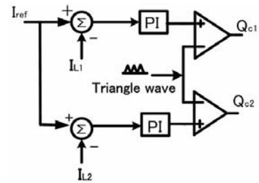
Fig. 8. Controller diagram of chopper circuit
