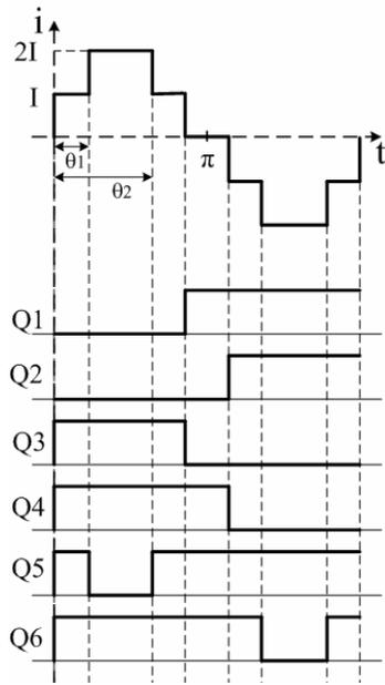
Fig. 5. Five-level current waveform generation
