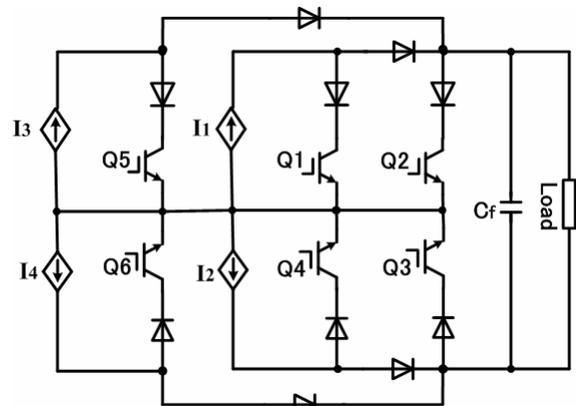
Fig. 4. Five-level CSI circuit ( $I_1=I_2=I_3=I_4=I$ )
