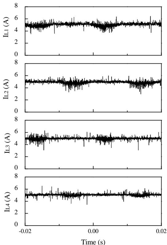
(b) Waveforms of DC current sources
