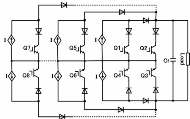
Fig. 3. Generalized configuration of proposed multilevel CSI
