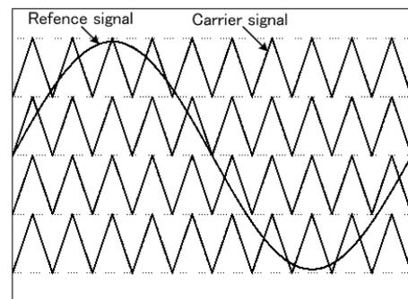
Fig. 10. Multi-carrier based sinusoidal PWM
