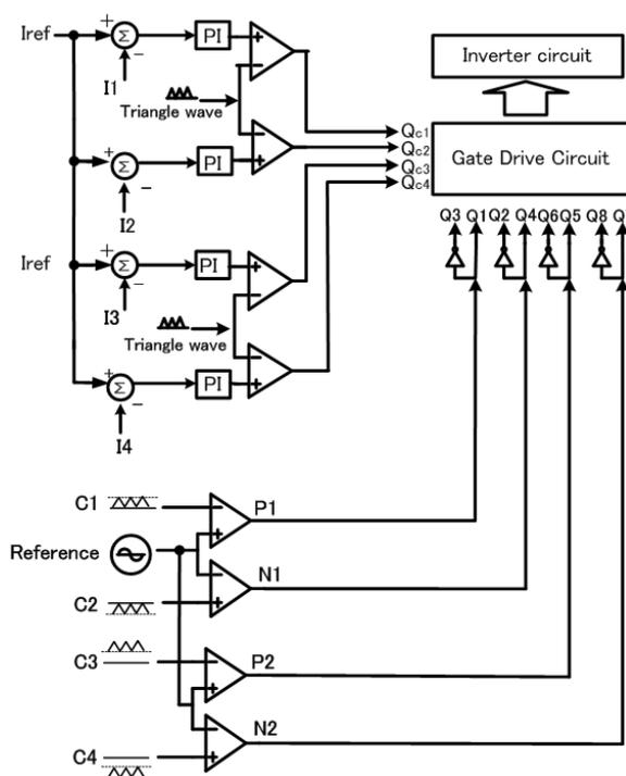
Fig. 11. Controller diagram of five-level CSI
