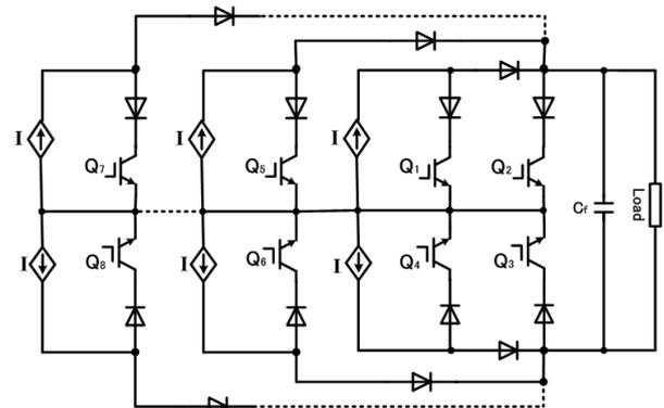
Fig. 3. Generalized configuration of proposed multilevel CSI
