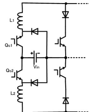
Fig. 7. Two-level CSI module with chopper circuit
