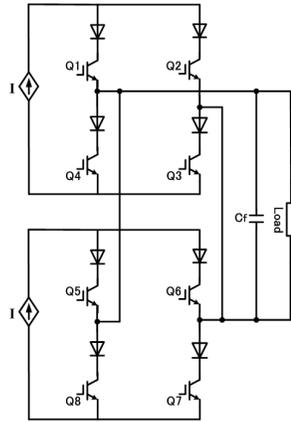
Fig. 2. Conventional multilevel waveform generation with parallel-connected H-bridge current-source inverters
