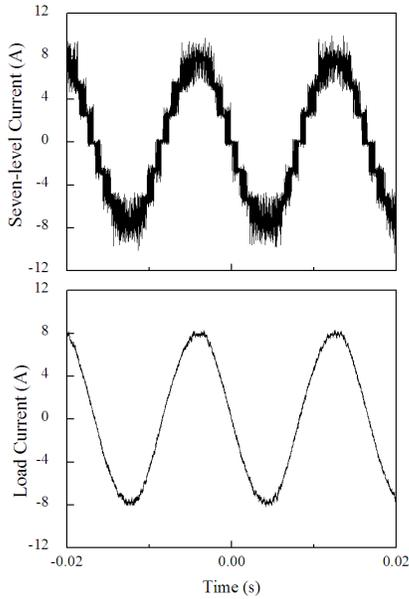
Fig. 13. Seven-level PWM output and load current waveforms of H-bridge inverter with doubly superposed DC current-source modules
