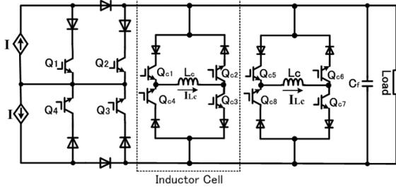
Fig. 6. Inductor cell based multilevel waveform generation applied to current-source inverter with common-emitter topology
