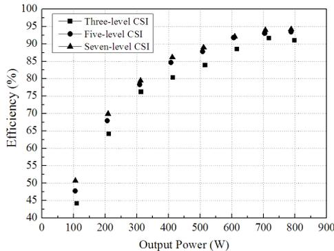
Fig. 14. Efficiency of H-bridge inverter with multiple superposed DC current-source modules
