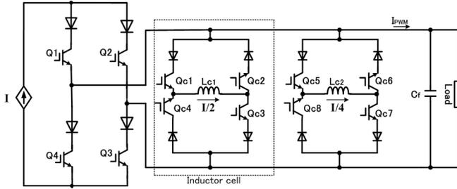
Fig. 5. Inductor cell based multilevel waveform generation applied to H-bridge current-source inverter
