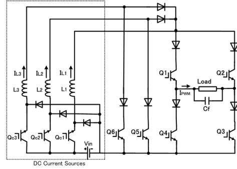
Fig. 10. Actual configuration of DC current-source modules
