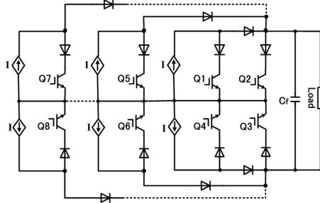
Fig. 11. Multilevel waveform generation with multiple symmetrical DC current source modules (extended fish bone structure based topology)
