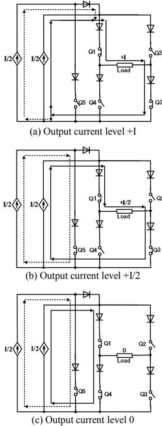
Fig. 9. Switching modes of five-level current-source inverter with superposed DC current source modules onto H-bridge
