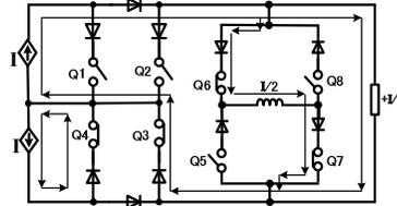
(b) Output current level +I/2 in energizing mode
