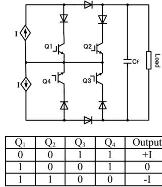
Fig. 3. Three-level current-source inverter with common emitter topology (fish bone structure based topology)
