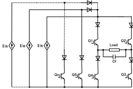
Fig. 8. Multilevel waveform generation with multiple DC current source modules superposed onto H-bridge inverter
