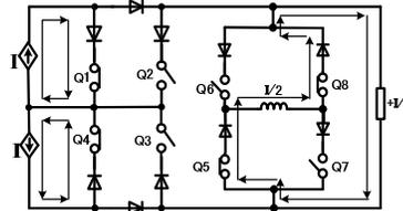
(c) Output current level +I/2 in discharging mode
