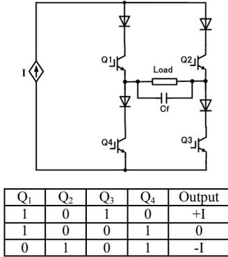
Fig. 1. Conventional H-bridge current-source inverter
