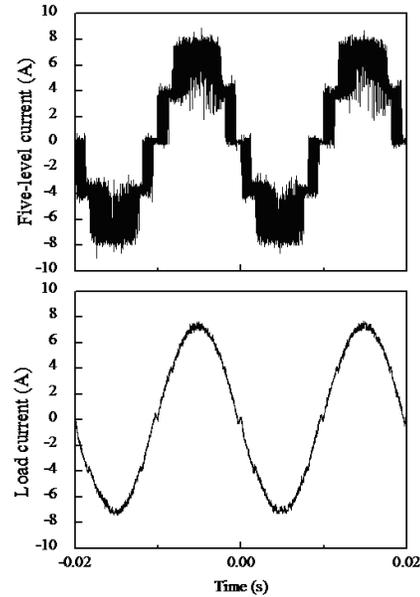
Fig. 12. Five-level PWM output and load current waveforms of common emitter current-source inverter with single inductor cell
