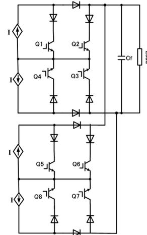
Fig. 4. Multilevel waveform generation with parallel-connected common-emitter current-source inverters
