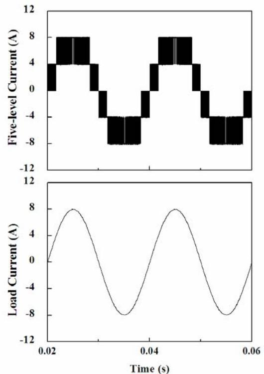
(a) Five-level and load current waveforms
