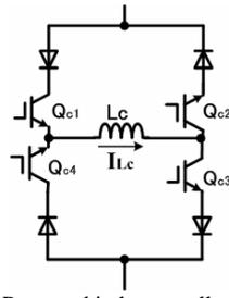
Fig. 2. Proposed inductor cell circuit
