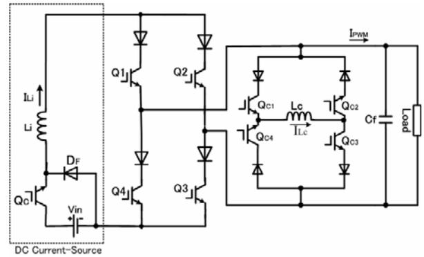
Fig. 5. Five-level CSI with chopper based DC current source
