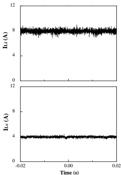
(b) Smoothing inductor current  $I_{Li}$  and inductor cell current  $I_{Lc}$  waveforms
