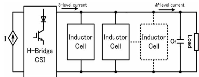
Fig. 1. Proposed configuration of multilevel CSI
