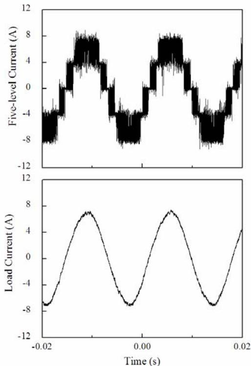
(a) Five-level and load current waveforms
