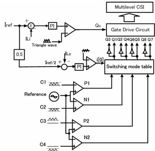
Fig. 6. Control diagram of proposed five-level CSI
