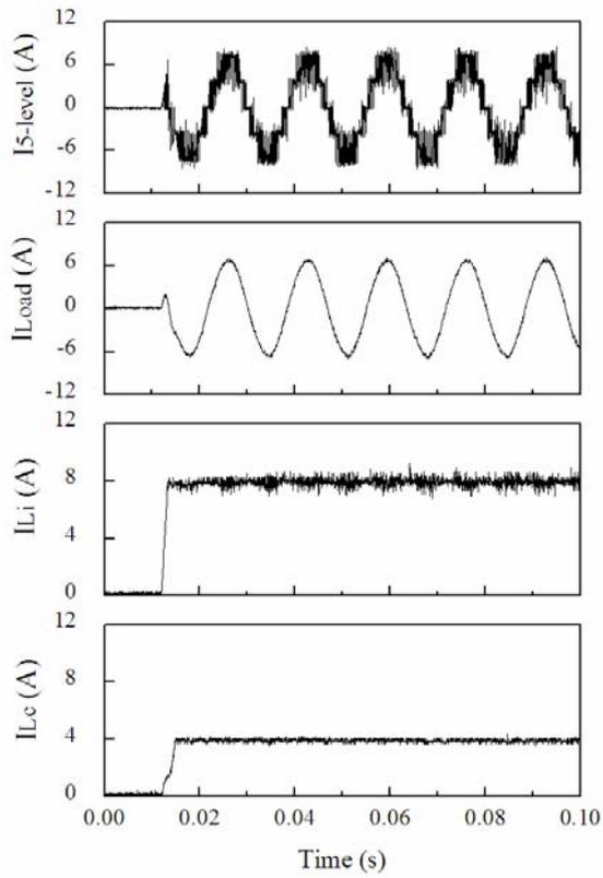
Fig. 15. Experimental waveforms of startup transient for five-level inductor-cell type CSI
