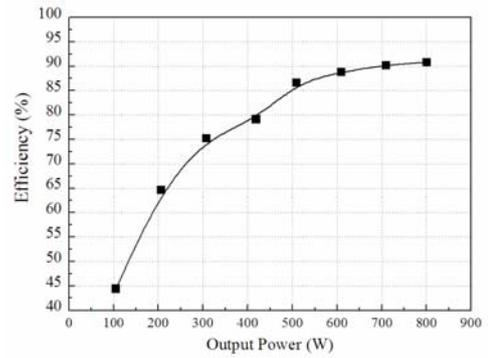
Fig. 17. Efficiency characteristics of five-level inductor-cell type CSI
