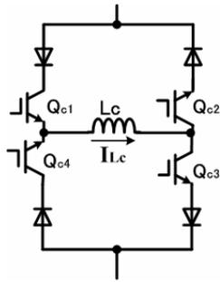
Fig. 3. Proposed inductor-cell circuits
