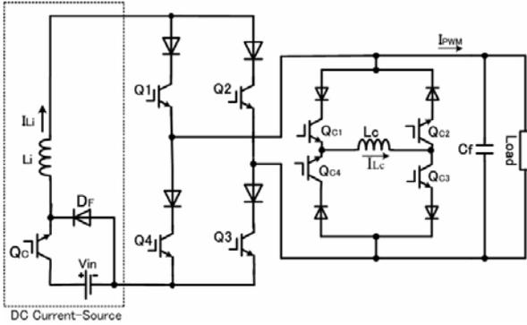
Fig. 10. Experimental circuit of five-level inductor-cell type CSI
