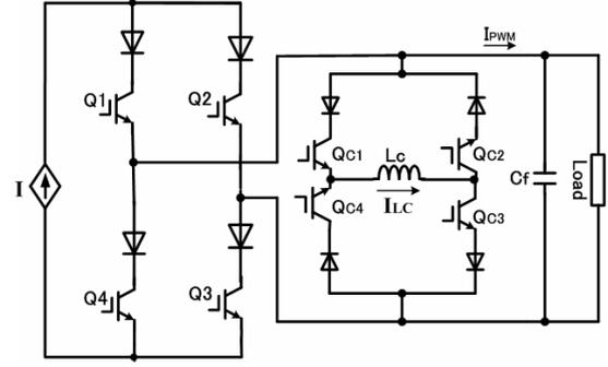
Fig.5. Five-level inductor-cell type CSI
