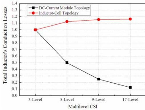
Fig. 14. Conduction loss characteristics of the inductors
