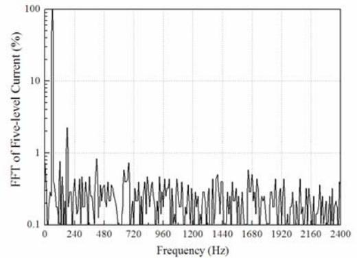
Fig. 19. FFT analysis result of five-level PWM current generated by five-level inductor-cell type CSI
