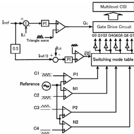
Fig. 12. Control diagram of five-level inductor-cell type CSI
