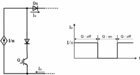
Fig. 7. Proposed DC-current module, and its typical output current waveform
