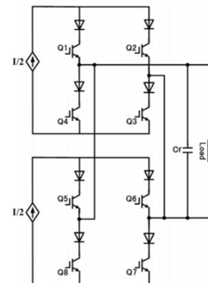
Fig. 1. Five-level paralleled H-Bridge CSI
