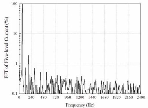
Fig. 20. FFT analysis result of five-level PWM current generated by five-level DC-current module type CSI
