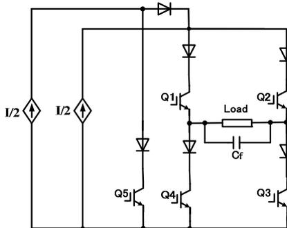
Fig. 9. Proposed five-level DC-current module type CSI
