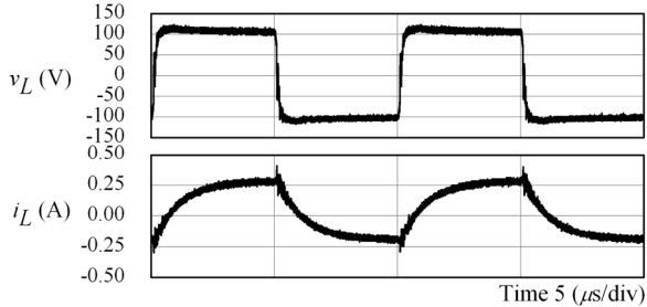
Fig. 13. Experimental waveforms of proposed inverter at 100-kHz output.
