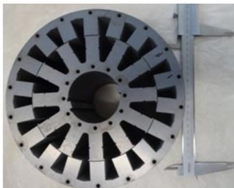
(a) Laminated rotor and stator cores.
