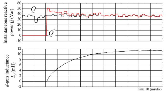
Fig. 8.  $d$ -axis inductance identification characteristic.
