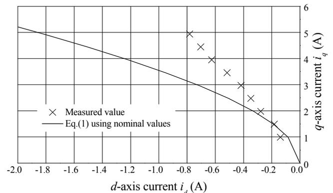
Fig. 4. Maximum torque per ampere control curves.
