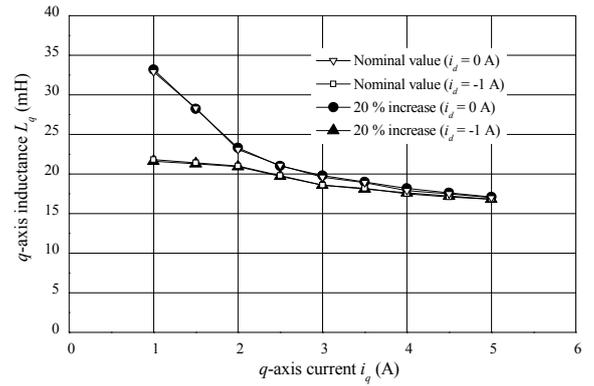
Fig. 12. Parameter sensitivity of winding resistance to  $q$ -axis inductance identification.
