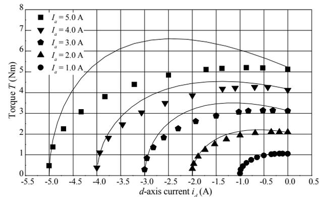
Fig. 3. Torque characteristic.
