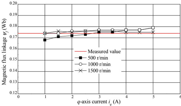
Fig. 7. Experimental results of magnetic flux linkage identification.
