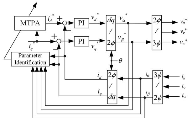
Fig. 13. Adaptive MTPA control system.
