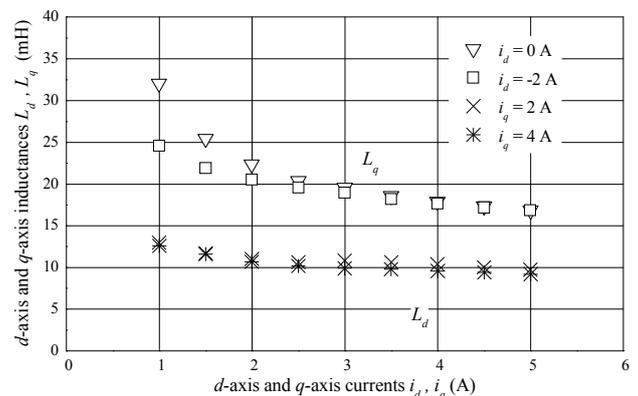
Fig. 1. Magnetic saturation characteristics.
