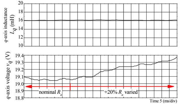
Fig. 11. Impact of winding resistance variation on  $q$ -axis inductance identification characteristic.
