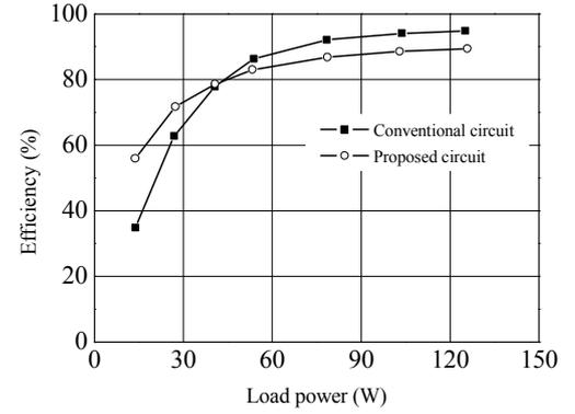
Fig. 12. Load power-efficiency characteristic
