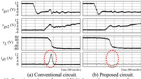
Fig. 10. Experimental waveforms of 50 % duty cycle operation of inverter at 14-W output.
