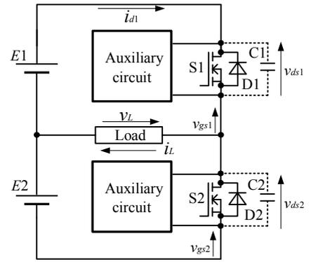
Fig. 7. Proposed inverter with auxiliary circuit.
