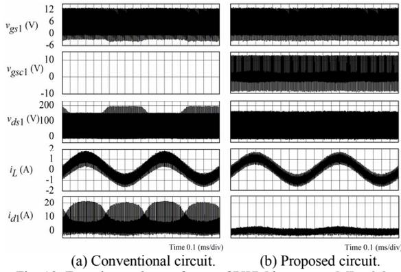
Fig. 13. Experimental waveforms of PWM inverter at MI = 0.2.
