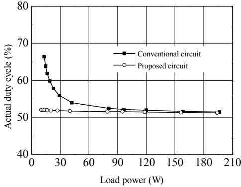
Fig. 6. Load power-actual on-duty cycle characteristic.
