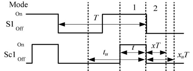
Fig. 2. Switching pattern of switching assist circuit.
