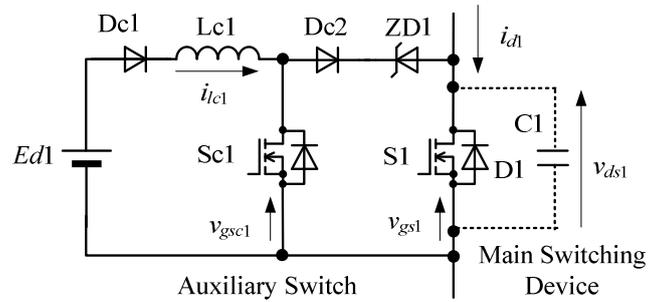
Fig. 1. Switching assist circuit fed by gate drive power supply.
