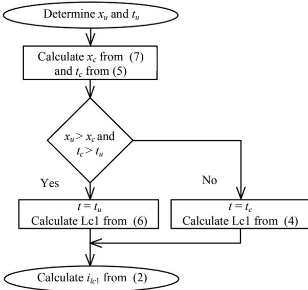
Fig. 3. Flow chart to determine parameters of switching assist circuit.
