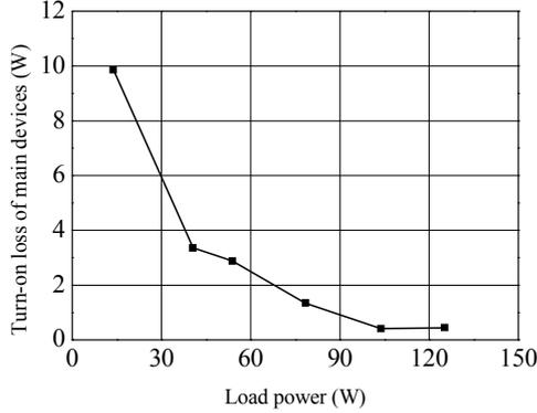
Fig. 11. Load power-turn-on loss of conventional circuit characteristic.
