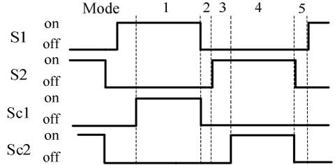
Fig. 8. Switching sequence of proposed inverter with auxiliary circuit.
