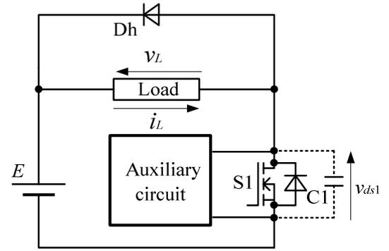
Fig. 4. Proposed buck chopper with auxiliary circuit.
