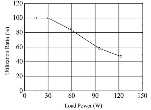
Fig. 16. Load power-utilization ratio characteristic.
