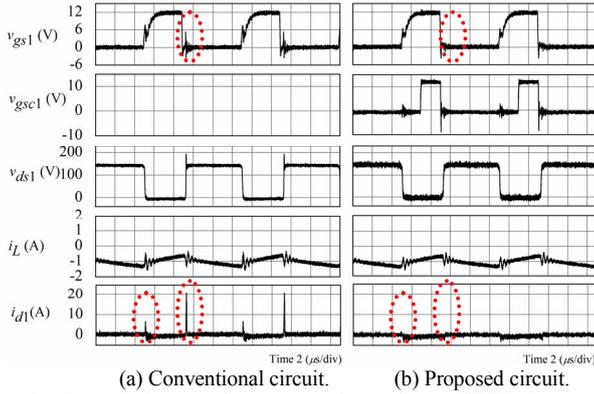
Fig. 14. Expanded views of experimental waveforms of PWM inverter at MI = 0.2.
