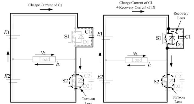
Fig. 9. Short-circuit current path of conventional circuit.
