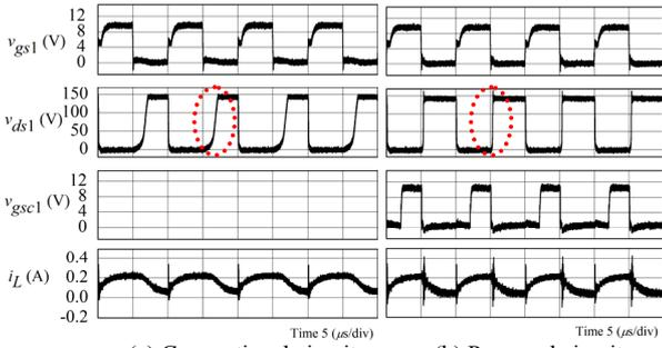
Fig. 5. Experimental waveforms of buck chopper.
