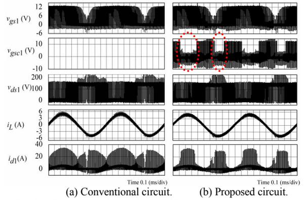
Fig. 15. Experimental waveforms of PWM inverter at MI = 0.9.
