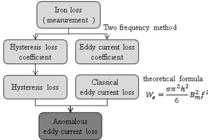
Fig. 1. Conventional anomalous loss separation method
