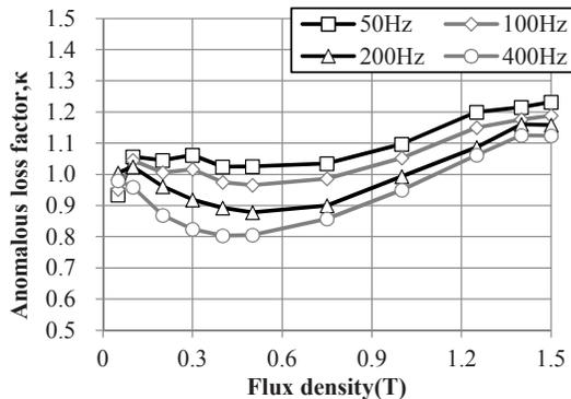
Fig. 2. Anomalous factor of 50A470 given by initial magnetizing curve
