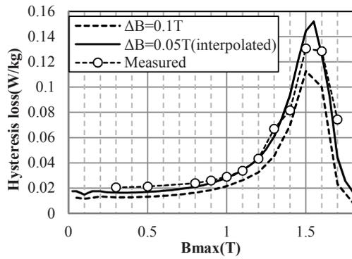
Fig. 7. Hysteresis loss of minor loop( $B_m:0.1T$ )
