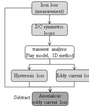
Fig. 3. Proposed anomalous loss separation method
