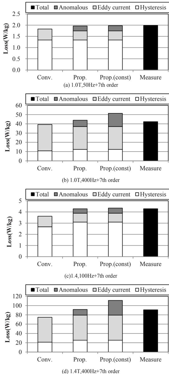
Fig. 11. Iron losses due to 7th order harmonics
