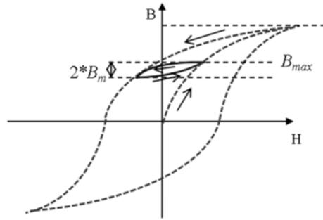
Fig. 6. Measurement of minor loop
