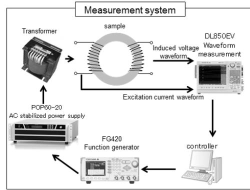
Fig. 8. Measurement system
