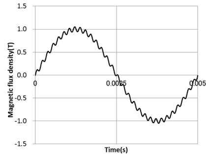
(a)Magnetic flux density waveform
