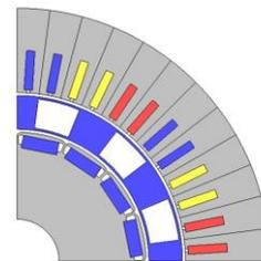
Fig. 1. Cross section of original prototype MMM.
