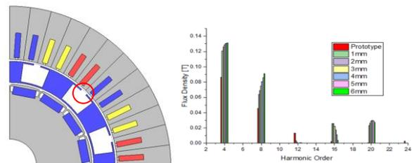
(a) Modified modulator. (b) Flux density FFT.
